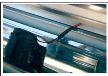
**Step 3**- Attach the wiring harness to the relay and get ready to pull wires. You should already have your lights mounted, so run the pair of Black and Red power wires out to wherever your lights are mounted. You can use a permanent connection by soldering or twisting the wires together and wrapping them in duct tape, or you can use a quick disconnect adapter in case you need to swap them around later.
