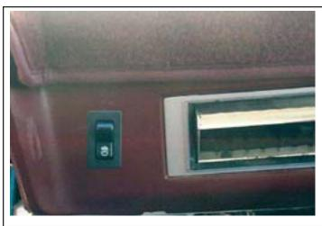
**Step 5**- The switch included with the wiring kit is an inline switch, which will just interrupt power to the relay, so you will have one wire to run to a 12 Volt Positive (+) source, and one to run back to the relay. Cut a hole in your dash by tracing the profile of the switch, or measuring the dimensions, then transferring the template to your dash. The switch just slides into place and locks itself down.
